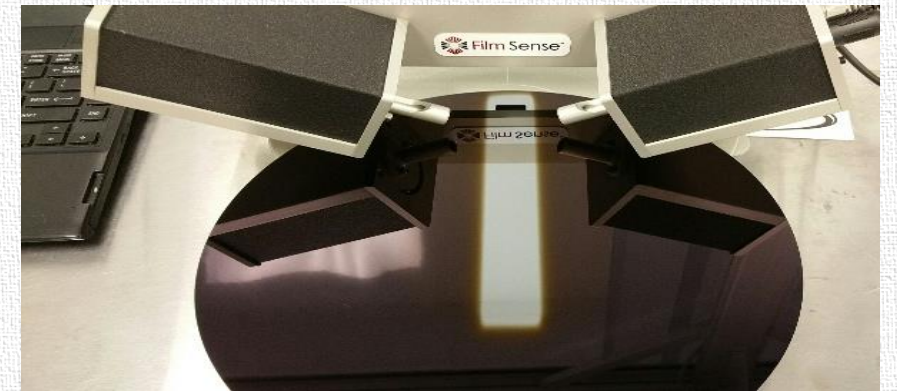
80Nm of amorphous carbon removed with Ontos AP Oxygen strip – room temperature
